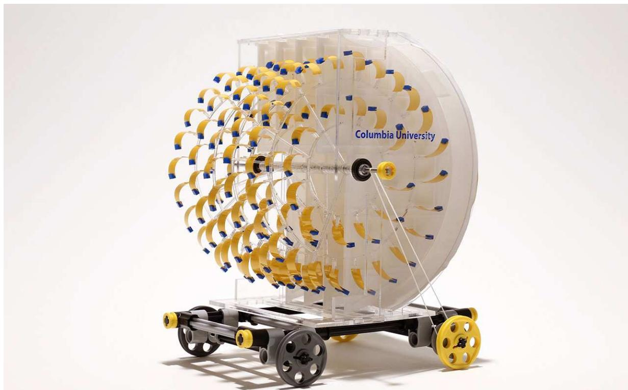
Evaporation engine prototypes use materials that expand and contract like muscles
